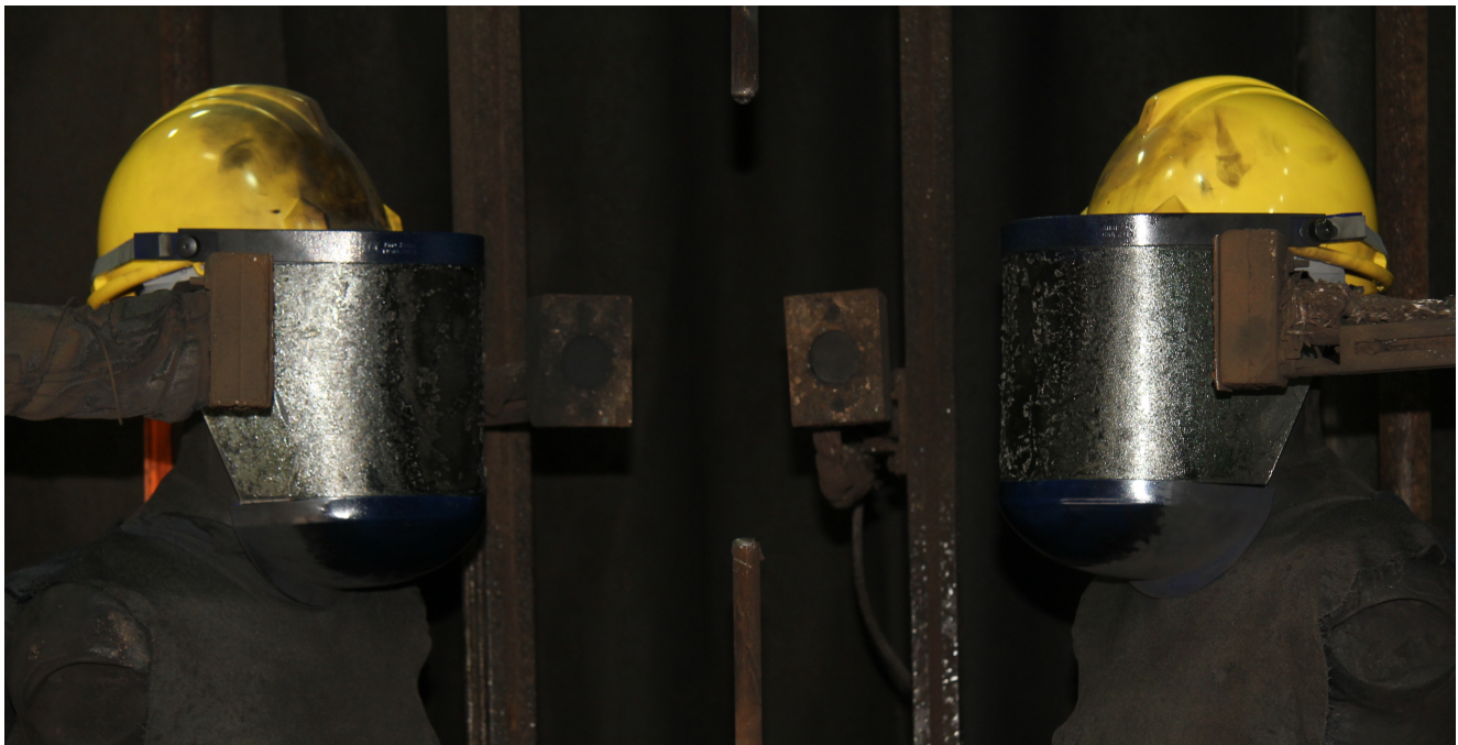
Figure 2. Faceshield after arc exposure at 19 cal/cm 2
